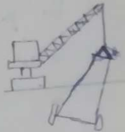
Upending by crane
